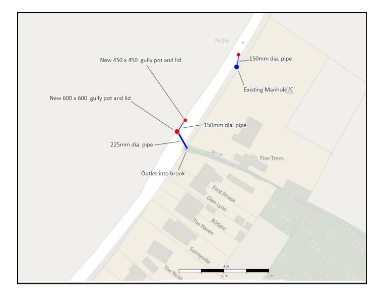
Please Install 1 no. new gully pot frame and lid and connect with 4.5m of 150mm dia. pipe to existing manhole C. Install a 450 x 450mm and 600 x 600mm gully pot frame and lid and connect with a 12mt length of 150mm diameter pipe. Dig trench across road and install a 225mm dia. pipe from the new 600 x 600mm gully pot to outlet into the existing brook that runs between Five Trees and First House. Reinstate and patch trench area 100mm thick. 60mm AC20 binder and 45/10 HRA surface course.
