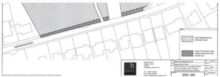
'The proposed works are to widen Newnham Road Hook, to facilitate access by a proposed new public bus service and footway along Newnham Road. See cross hatching on plan above.
