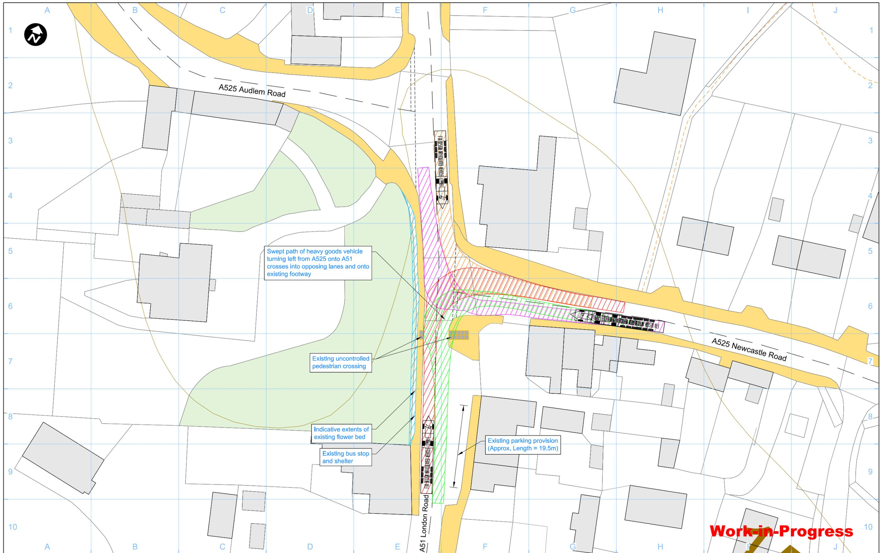
Swept path of heavy goods vehicle turning left from A525 onto A51 crosses into opposing lanes and onto existing footway
