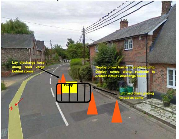
*Image D – 12" pump and tractor deployment location outside 'The House', view looking downstream to the south-west.*
