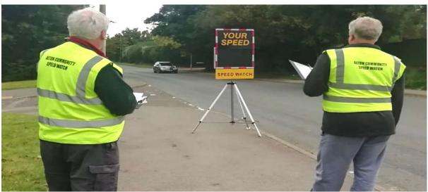
Figure 9 – Example of mobile VAS displaying vehicle speed
