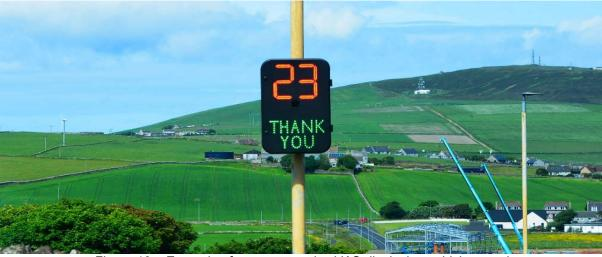
Figure 10 – Example of more expensive VAS displaying vehicle speed
