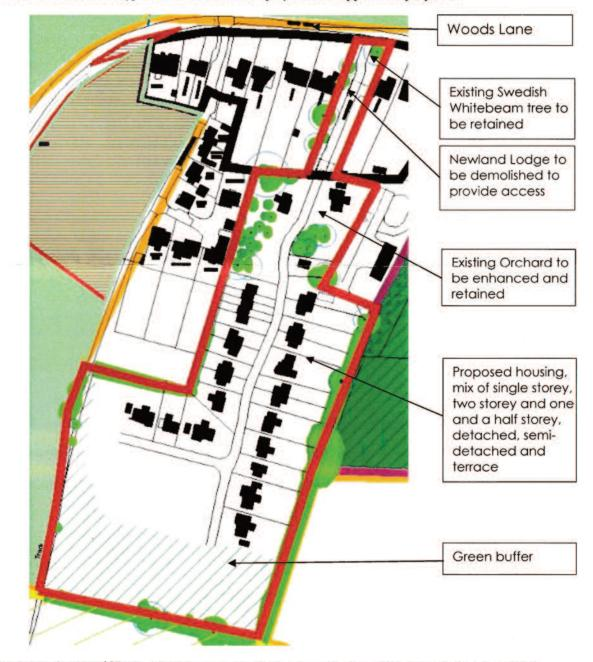
Fig 4 – extract of drawing number 1543/SP-02 – showing proposed housing layout, existing trees will be retained and enhanced and south of the site will be left free from development and will incorporate biodiversity enhancements
