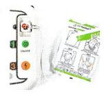
Stick pads to casualty as illustrated on the pads. The visual indicator on the device will also light up to illustrate where to stick the pads.
