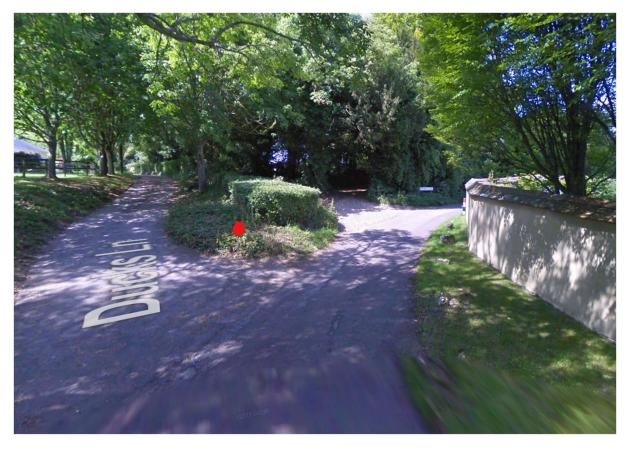
Install 1 X FORD sign (FIG 554 @ 600mm) and 1 X 350 Yards plate (FIG 572 with X-height of 62.5mm) in direction of Ford.
