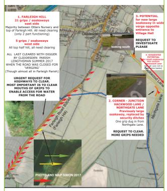
'GRIPS': Channels cut through a grass verge (specifically for the purpose of draining water away from the highway).'
