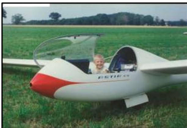
Sailplanes rely on high-aspect ratio (wide but narrow) wings for lift; weather conditions too affect the ability to gain height and remain aloft. Without an engine, much depends on pilot skill, prowess and an understanding of prevailing weather and atmospheric conditions that play such a vital part in the whole proceedings. Pilots must, for example, take advantage of thermals, columns of rising air, if they are to soar and travel hundreds of miles.
