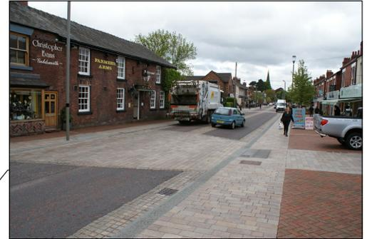
20MPH ZONE SHARED SURFACE VILLAGE CENTRE TO INCLUDE BLOCK PAVING AND MINIMAL ROAD MARKINGS
