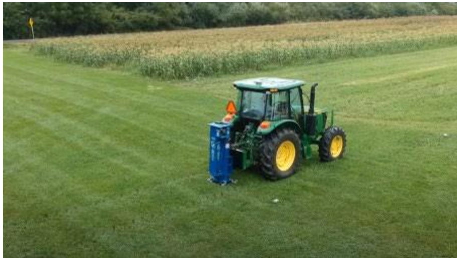
Figure 3 'Weight Drop' mounted on a tractor operating 'cross-country'
