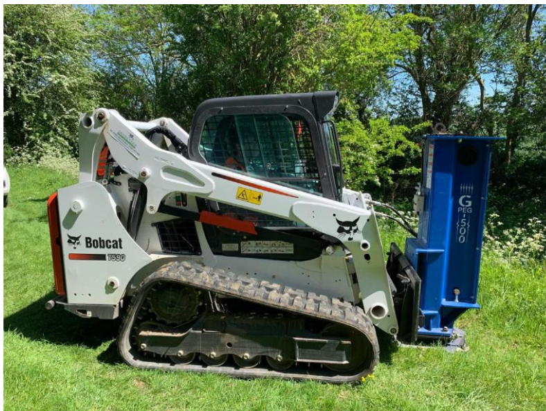
Figure 4 'Weight Drop' mounted on a tracked bobact operating 'cross-country'
