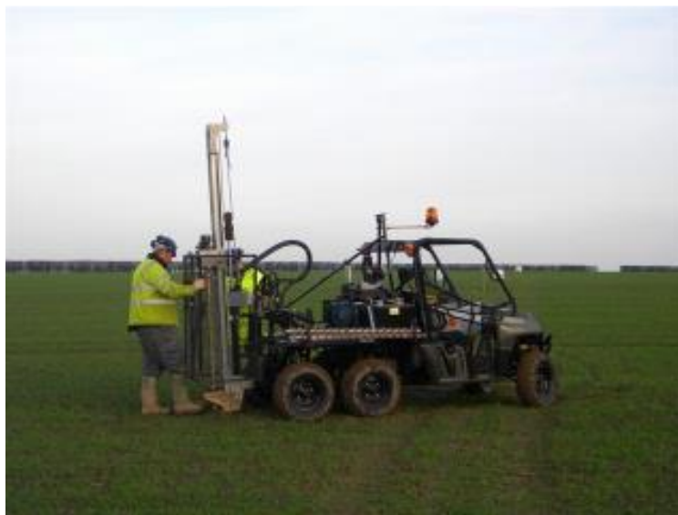
Figure 5 'Polaris' 6WD quad based auger unit
