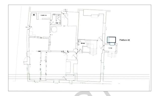
This solution had previously been discounted as unfeasible, partly due to the surface and steepness of the driveway from the High Street. However, SG will draw up a plan to raise the level of the porch floor, re-hang the main door to open outwards and install an enclosed lift.
