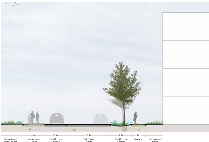
Figure 12 - Commercial Loop Section
