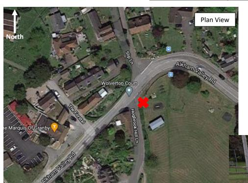
New signs to be installed on new post (3/1 & 3/2) behind existing name plate and bush, in south-western grass verge. Signs to be mounted so they are clearly visible to traffic travelling along Alkham Valley Road. Please refer to sign schedule and attached sign designs.
