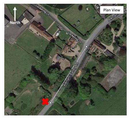
Existing sign to be taken down and set aside (TD4/1). Existing signs (TD4/2 & TD 4/2) and post to be taken down and tipped. New and existing sign to be installed on new posts (6/1 & 6/2) in northern grass verge where existing signage is located. Please refer to sign schedule and attached sign designs.
