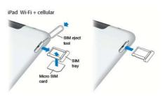
SIM into the tray (it can only go in one way) and put it back into the iPad. Turn your iPad on and you will see the Wi-Fi bars being displayed in the top left corner, like the ones you see on your phone when you have a signal.
