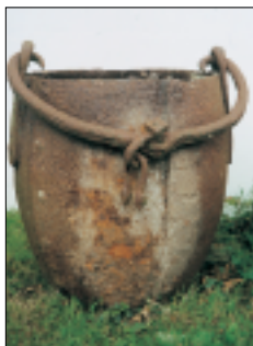
A wrought iron kibble. The design is attributed to Richard Trevithick.
