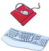
**Mouse:** Acts as a handheld pointing device and controls the actions of that blinking item on your computer screen known as a *cursor*.
