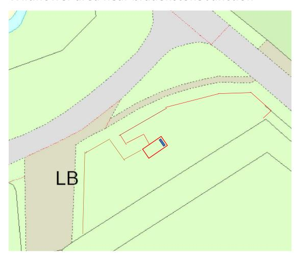
Red line new barrier 400mm high constructed with 75mm x 75mm 2.4m lengths on 100mm x 100mm posts.
