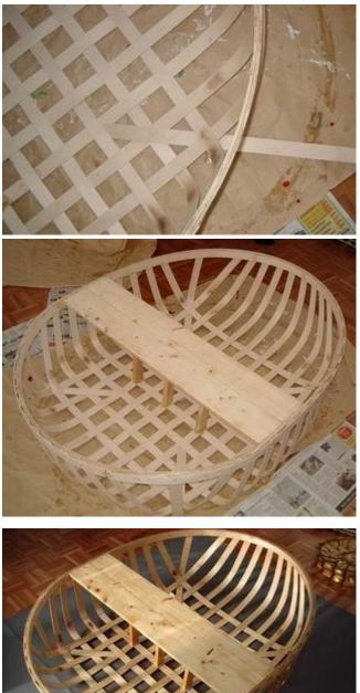
Every corner of the coracle will have an extra corner lath. Each corner lath touches three crosswise and lengthwise lath crossings. Between the laths, on the inside, and on the outside.
