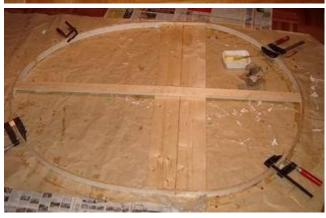
A second and third layer of laths are wrapped on the first layer, glued to previous layers, the ends of the laths are nailed to the ends of the seats again.
