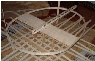
When the seat-gunwale is positioned on top of the basket bottom and vertical supports, the front edge of the seat comes directly above the middlemost crosswise lath. The supports land on the next crosswise lath, the mid support on the mid lengthwise lath, the others on the third and seventh lengthwise lath (sounds a lot more complicated than it is ;-). The ends of the supports are glued and screwed to the lath crossings.
