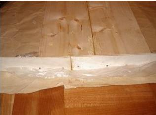
The ends of the laths are glued and nailed (or screwed) into the ends of the seat. The seat and gunwaler are now upside down. When turned right side up the top of the seat will be flush with the top of the gunwale.
