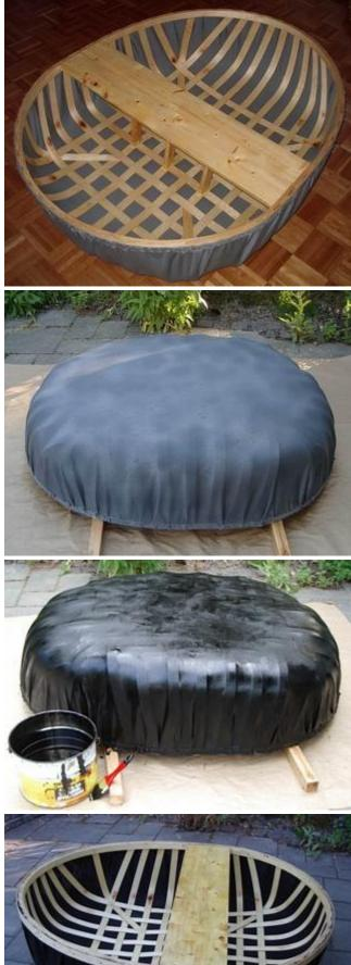
The edge of the fabric cut short, then folded out to double thickness, and stapled to the gunwale.
