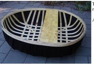
Three coats of the bitumen emulsion, and one more lath ring to protect the outside edge of the gunwale.
