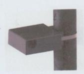
Auto Speedwatch (illustrated left) is a solar-powered device that captures images of the rear of speeding vehicles and sends these, together with speed and registration data for checking, to an Internet Dashboard. Community Speedwatch volunteers then need to check and verify the information for onward transmission to the Police via the Community Speedwatch system.
