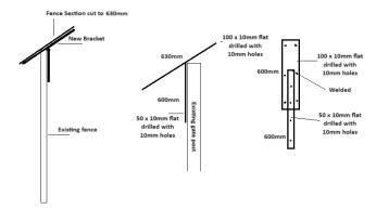
**Quote A:** Supply & fix 868 Mesh Panels (to match existing fence) 630mm x 2506mm L - Green RAL 6005 – with purpose built fixing brackets. Comes with corner brackets and mesh panel connectors. Price includes access equipment for installation. £15,000
