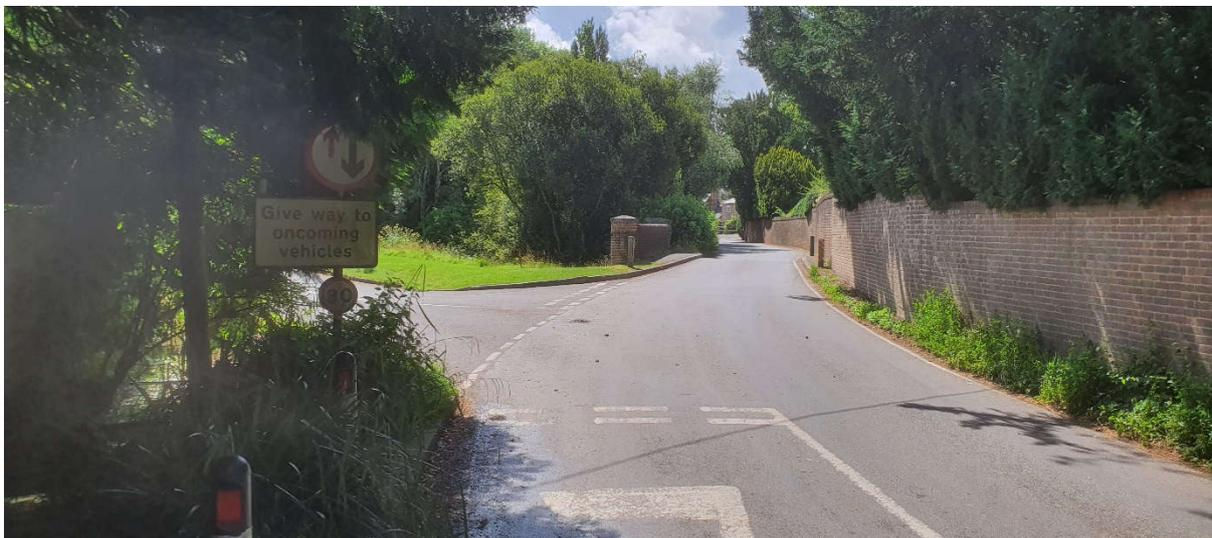
There are 300mm 30mph repeater at infrequent intervals throughout the village. Without regular repeater signs along a route the road is assumed to be the national speed limit for a single carriageway. However, some of the existing repeater signs are not conspicuous due to the size of the signs and their location. Vegetation obscures some of the signs and the condition is poor for several of the signs. As a result of this drivers do not have a regular reminder of the speed limit.
