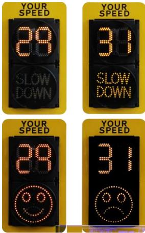
230V mains or 12V powered (Depending option ordered), Mini 300 SPEED DISPLAY, polyurethane bodied modular sign c/w a Yellow Non-Reflective border and "YOUR SPEED" text The Inter-active sign will display a 200mm real-time illustration of the approaching speed of an oncoming vehicle. When exceeding a pre-set threshold limit, the sign will display a "SLOW DOWN" safety message in Amber LED's. Or a Sad/Smiley face depending on the option you choose.
