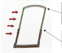
Joints between frame & roof structure not designed to resist lateral loading.
