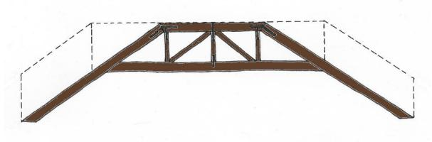
Figure 7 – 'A' shape Howe truss
