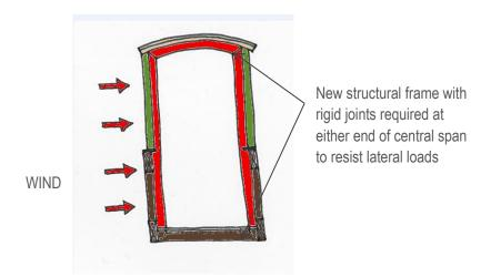
Fig.9 Strengthening required to resist lateral loads
