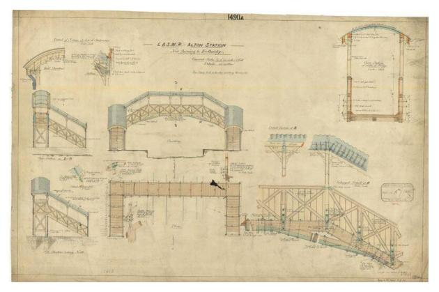
Figure 1 – LSWR drawing of planned cladding and roof at Alton.
