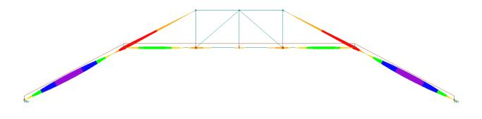
Fig. 8 Fully loaded model showing locations of maximum bending moments
