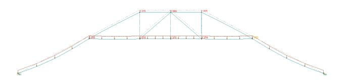
Fig. 7 Deflected shape of fully loaded bridge showing vertical deflections of less than 2mm
