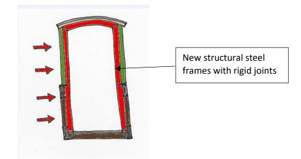
Figure 9 - Diagram of stiffening from the Integral report
