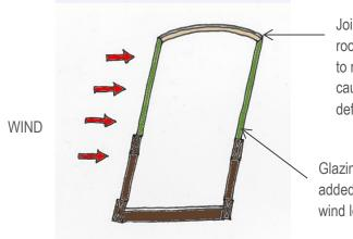
Joists between frame and roof structure not designed to resist lateral loading causing excessive deflection
