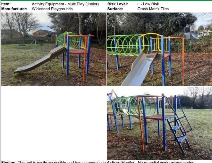
**Finding:** The unit is easily accessible and has an opening in **Action:** Monitor - No remedial work recommended the barrier to steep play elements in excess of 500mm in contravention of BS EN 1176 Part 1
