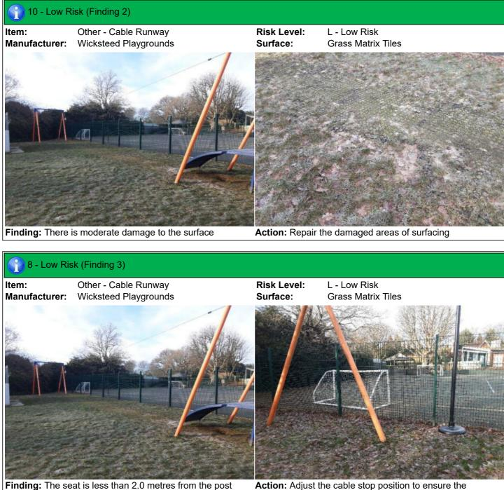
**Finding:** The seat is less than 2.0 metres from the post when extended at 45 degrees at the end of the area of travel minimum distance is maintained and does not meet the requirements of BS EN 1176 Part 4
