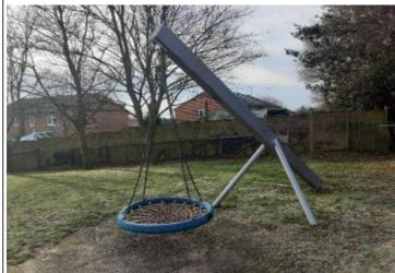
Finding: The seat clearance from finished surface level to the underside of the seat is too low and does not meet the requirements of BS EN 1176 Part 2 (400mm minimum clearance required from rigid part of seat in most onerous position)
