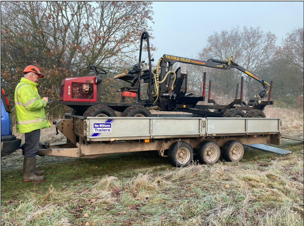
The eight-wheeled 'forwarder' can grab and carry timber off site without causing any damage or rutting of the public bridleway, meaning walkers and riders can continue to enjoy using the bridleway to pass through Line Bank and on to Idle Stop without getting stuck in the mud.
