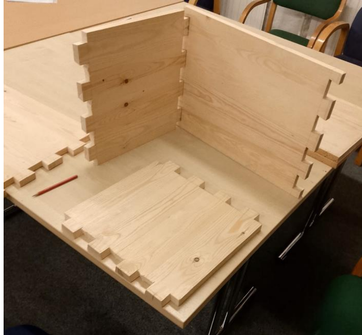
Joints : Delia's box is for Lego bricks A Wednesday Woodwork project
