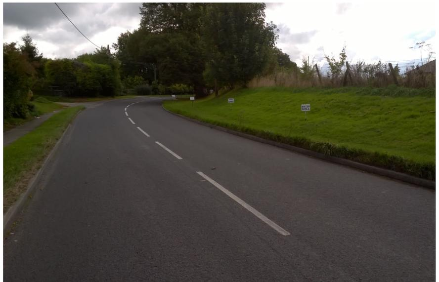
The removal of the carriageway center lines increases the risk of head on collisions around bends.
