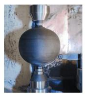
Figure 1 Taylor bowl being shaped by a lathe [6]
