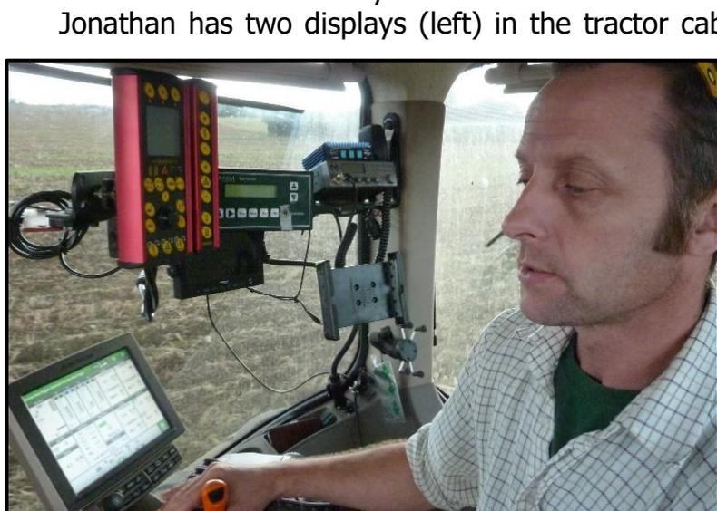
Jonathan has two displays (left) in the tractor cab. One screen depicts the field and the route the tractor is following. The system automatically accounts for different implements and widths and can plot the most efficient path to take. When first 'mapping' a field Jonathan will drive round the perimeter using a headland of some 9 to 20 metres, depending on implement.
