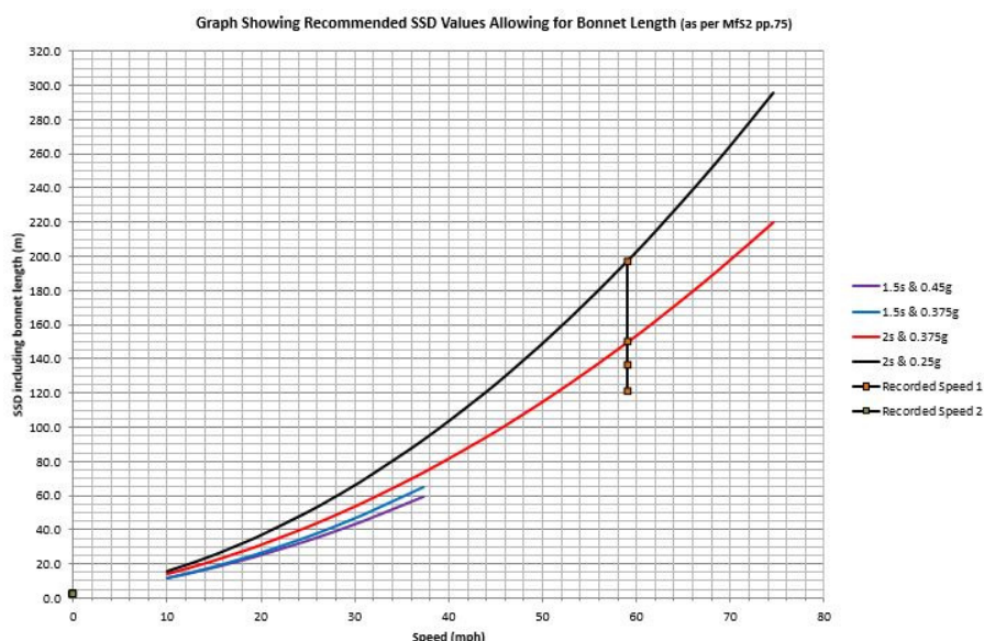
Figure 2: Manual for Streets 2 Visibility Graph with 150m SSD
