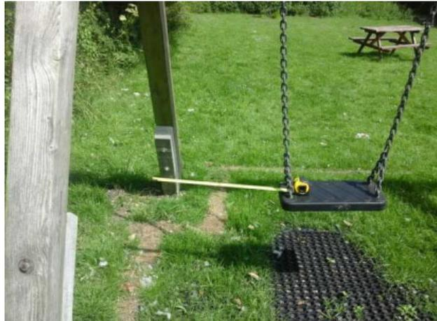
**Finding:** The seats are too close to the frame as defined in BS EN 1176 Part 2; this is a low risk failure and no remedial action is required
