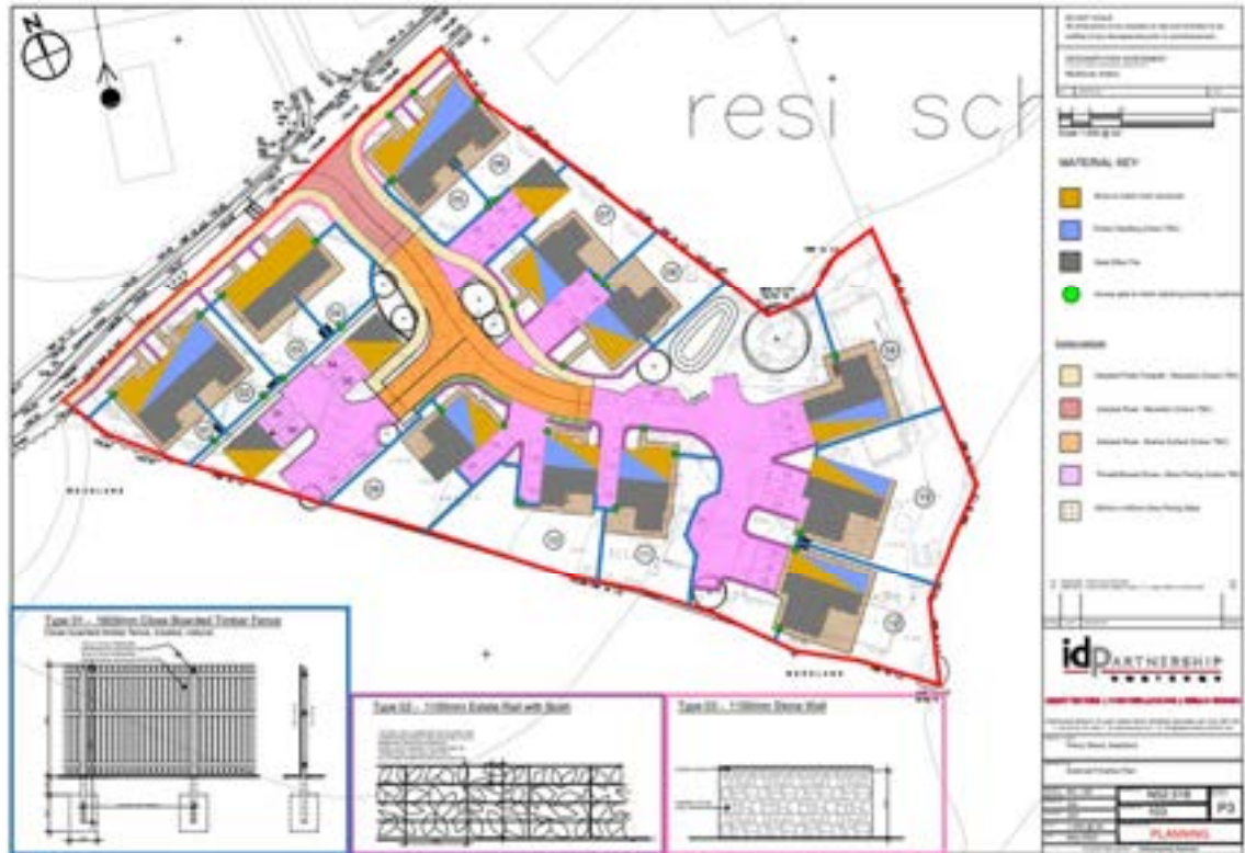
Figure 5.2 External Finishes and Boundaries
