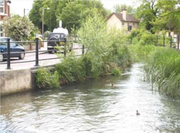
Photo 22: Wetland vegetation is encouraged to provide habitat and to screen the steel sheet piling, which forms the river bank in Bishopstoke
