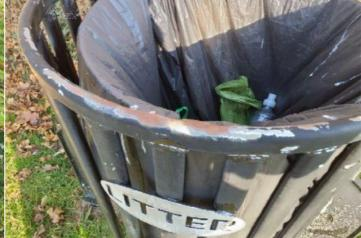
worn exposing the metal underneath which is rusting
