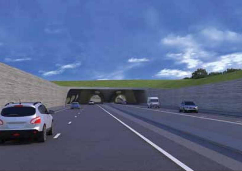
Figure 5.34: Driver's view of canopy with ventilation outlets - entering
