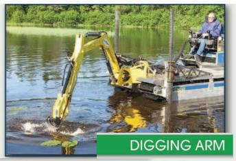
This attachment is made of high tensile steel which keeps the weight low without compromising on strength and has a maximum digging depth of 3m.
