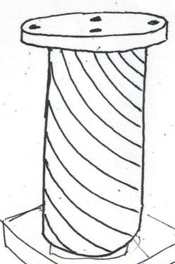
The top could be glued in place with water proof resin glue:
